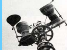
Figures 1-2. The BNSS astrophotograph (right): Ernstar aperture is 13.5 cm, focal length 24 cm, scale 859"/mm, FOV 28". BAM014B Plate centers distribution for 5845 plates included in the WFPDB (left).
