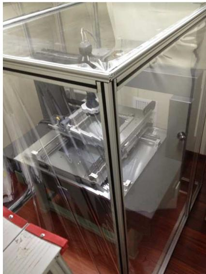
**Fig.2** Digitizer is covered with a customized plastic sheeting room to reduce the impact of the airflow from indoor air conditioning.
